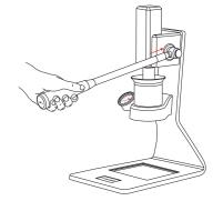
①. Take out the pull rod and install the metal washer.
